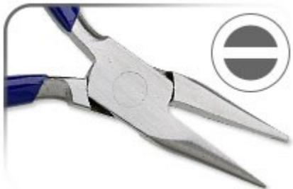
**Chain-nose pliers** have jaws that are flat on the inside and round on the outside. The jaw tapers from the joint to the tip. The flat inside of the jaw allows for a secure grip on small findings and pieces, such as when opening a jumpring. The curved outside is helpful in making small loops and curves on wire.
