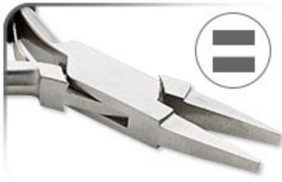
**Flat-nose pliers** are flat on the inside and outside of the jaws and don't generally taper as much as chain-nose pliers. Use these to securely hold findings, such as when opening a jumpring. Because of the strong grip without marring or scratching these are useful when drawing or pulling wire. The rectangle shape of the jaw lets you create sharp corners more easily than when using chain-nose pliers.
