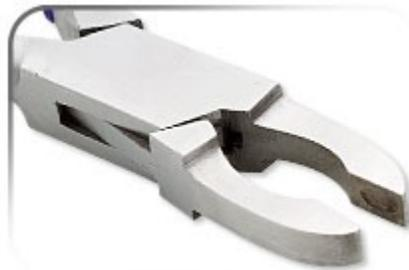
**Loop-closing pliers** smoothly close loops, jumprings, bracelet links and more without causing a shape change. The jaws have a groove which allows for the curvature of differently sized loops and prevents distortion and scratching.
